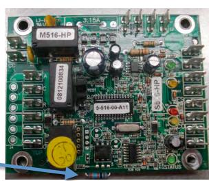
For units already installed that exhibit this condition, the picture below shows an alternate method that achieves the same results. Units shipping from the Greenville warehouse will have the alternate design as shown below; units shipping from Mitchell have the new lockout board, as shown above. Eventually, all units will be shipping with the new lockout board, and will not have a resistor at the terminal strip.
